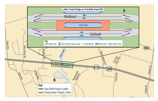
Roadway map shows the planned eastbound and westbound lane shifts before and after the Lofton Creek Bridge shifting traffic on A1A/State Road 200, weather permitting.
