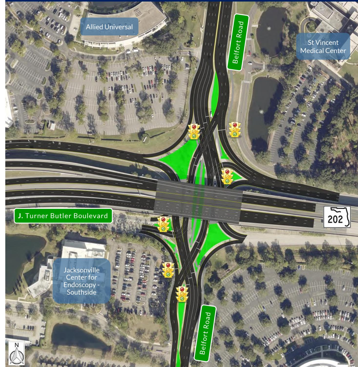
The J Turner Butler Boulevard at Belfort Road interchange will be converted to a Diverging Diamond Interchange as shown. Belfort Road will be widened to accommodate two through lanes and two left turn lanes in both directions. The through movement will be eliminated at the exit ramps, and an additional right turn lane will be provided for the westbound exit ramp.
